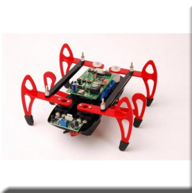
3 Servo Arduino based Hexabot
